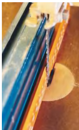
▲ The fence is brought up and adjusted so it is parallel to the Buddy
